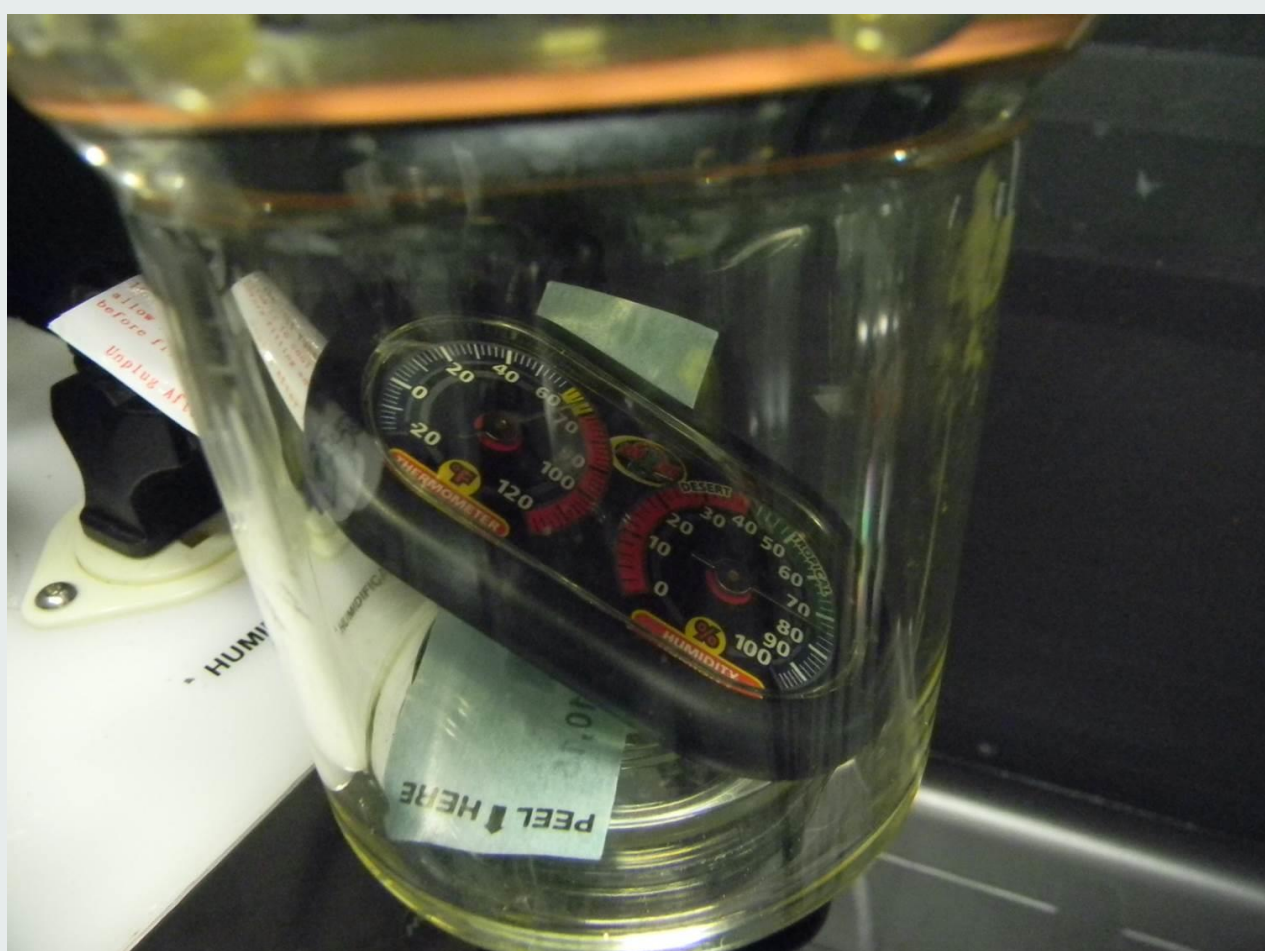
BI's within the Temp/RH and BI Holder (for decontamination verification) and attach to Return Hose
